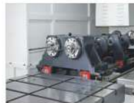
双坐标双主轴结构 Double coordinate double spindle structure
