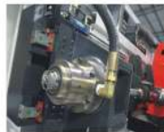
三轴枪钻、BTA一体结构 Three axis gun drill and BTA integrated structure
